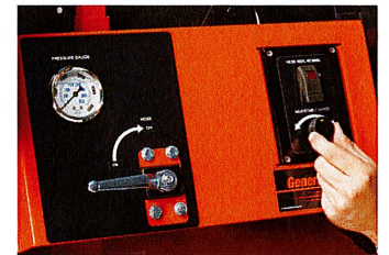
Easily accessible Variable Speed rewind control, along with pressure gauge and output valve mounted between hose reels.
